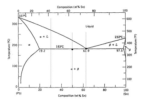
(a) eutectic mixture: Pb-61.9wt%Sn at T = 183°C.
